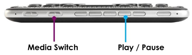
You can open the DAISY Player by moving the media switch to the center position, labeled "DAISY", then pressing the Play button on the front panel.
