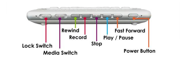
On the far left of the front panel is located a 3-position slide switch. In the "Lock" position, which is furthest left, all keys on the top and front panel are locked. In the "Audio" position, which is the center switch position, then the top panel will be locked, but the front panel will be unlocked. In the "Unlock" position, which is the furthest left switch position, all keys are unlocked.
