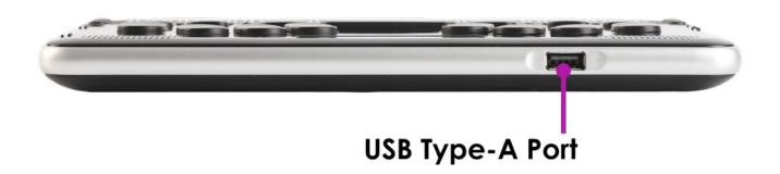
The rear panel of the BrailleSense 6 contains another USB A host port, for connecting drives, keyboards and mice, cameras, printers, audio gear and other compatible USB peripherals.
