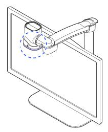
2. Raise the locking lever fold the camera arm.
