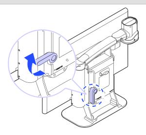
2. Pull up on the camera arm to adjust the height.
