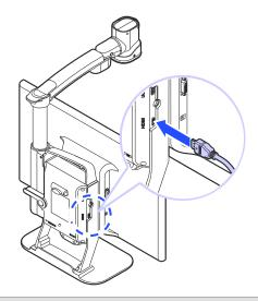
2. Connect the HDMI / DVI adapter to the computer monitor port.
