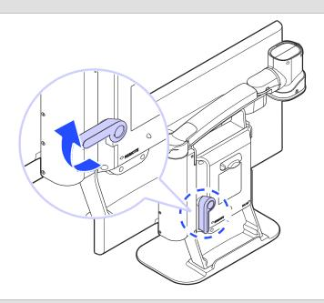
2. Pull up on the camera arm to adjust the height.
